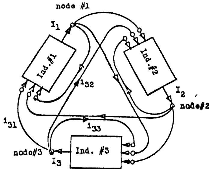
A node is a symbol of collection and distribution of flow. Node #3 receives from industry #3 and distributes to industries #1 and #3. If industry #3 manufactures chairs, then a flow from industry #3 back to industry #3 simply indicates that industry #3 is using part of its own output product, for example, as office furniture. Therefore the flow may be summarized by the equations:
